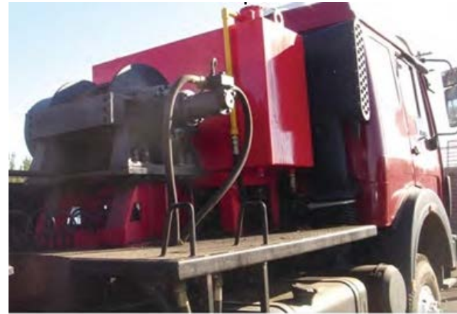
40 tons Winch on Heavy Duty Truck at Oilfield
