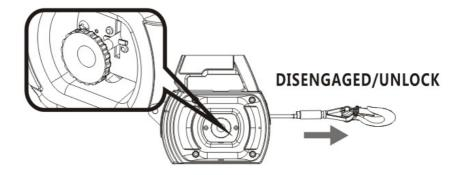
Pull out the knob and turn it counterclockwise to have the clutch fully engaged again.
