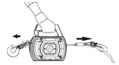
**Spooling with an Assistant:** Have the person handling the rope hold the hook strap and walk the winch rope away from the winch while spooling out the winch rope.
