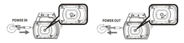
The drill/driver's speed trigger controls the power and speed of the power-in and power-out operation. To turn the winch ON,depress the drill trigger.
