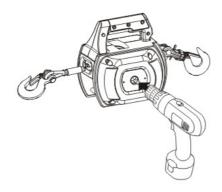
(2) Secure the chuck of your drill around the driver shaft tightly to avoid the drill slipping off the shaft.
