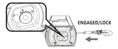
The clutch will not disengage the gear train if there is tension on the winch rope greater than 15lbs.
