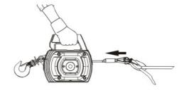
(3) Arrange the winch rope so it will not kink or tangle when powering-in by keeping tension on the winch rope.
